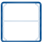
SECTION A-A LINE POST STIFFENER ALUMINUM INSERT
